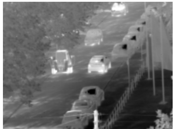
Fig. 3: IR-scene taken by a QWIP-camera operating in the LWIR.
