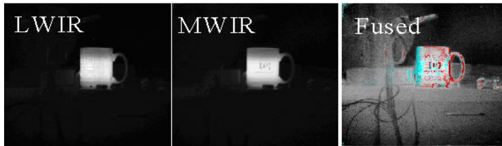
Figure 2. Image of a coffee mug with bead-blasted and printed lettering. At right is a color image fusion of the LWIR and MWIR images.
